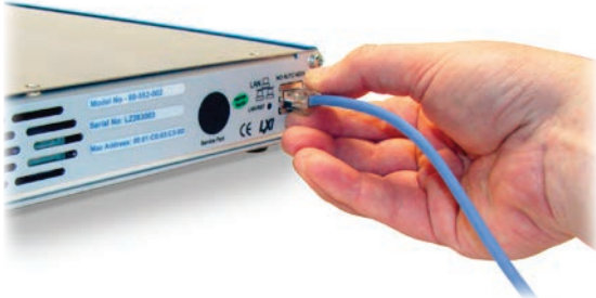
Connect one end of the Ethernet Cable to your LXI Switching Device
