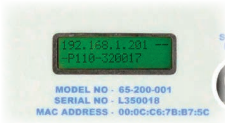
IP address display on the rear panel of a newer LXI Switching Device
