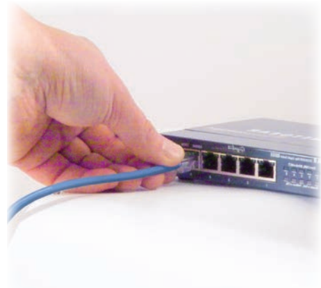
Connect the other end of the Ethernet Cable to a hub or switch
