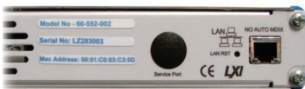
MAC address label on the rear panel of your LXI Switching Device
